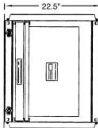
Sureseal Housing with 12" Rigid-Air and PrePleat 40
